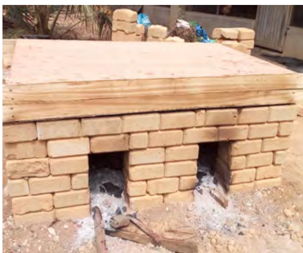
Chorkor oven (oven used for fish smoking) This picture shows trainees participating in fish processing at Doctor Fish Agric Consult Training Center, Delta State.
